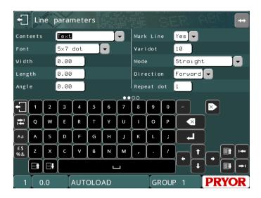
Press the buttons to change the line's data that is displayed. The line number is shown in the bottom left of the screen.
