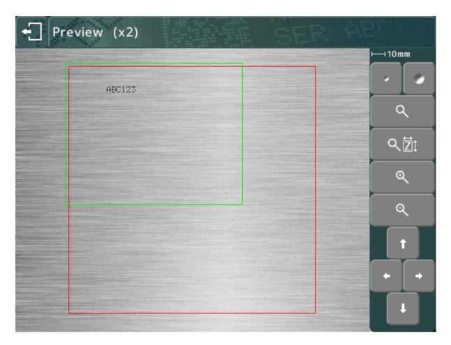
The mark may be very small. To zoom in use the cursor keys to move the green box over the text and press the button. Press ESC to go back to the zoomed out view.
