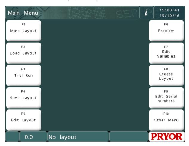
Menu options can be chosen by pressing on the menu buttons on the touch screen. If a keyboard is connected, options can be selected from a menu by using the cursor up/down keys to highlight the required option and then pressing ENTER or by pressing the appropriate function key shown screen.
